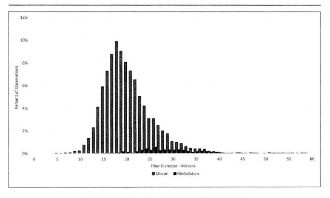
Test Performed According to Method AS/NZS 4492.5:2000
